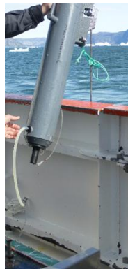
Figure 8. Silicon tube used to decrease organism loss and damage when water samples are collected into amber glass bottles from Niskin bottles.
