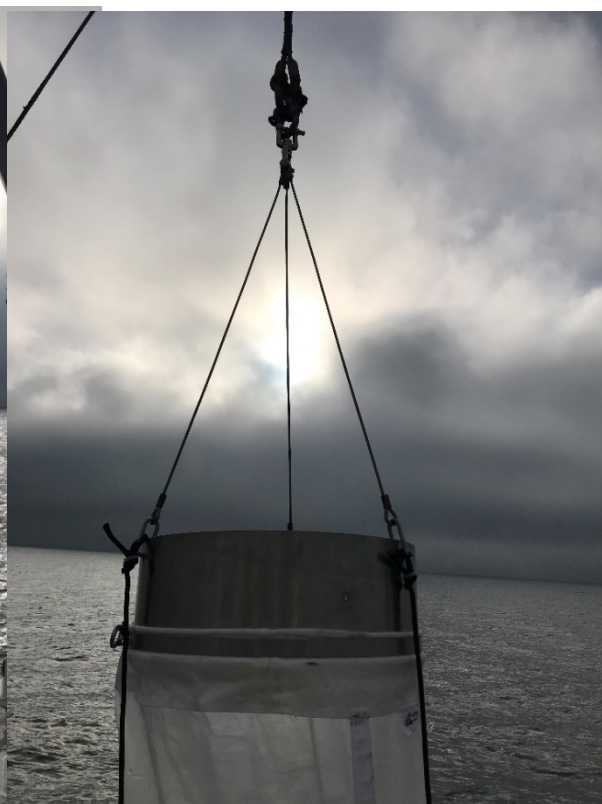
Figure 2: Close up of net drum, bridle and shackles linking to winch rope
